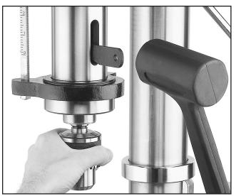
Figure 32. Using drift key to remove arbor.
